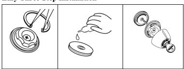
1 Assemble Anchor Bolt using retaining ring pliers. Drill 5/16" diameter hole in desired location.
